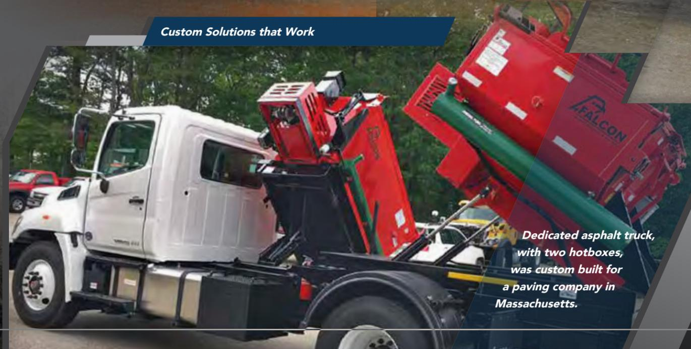
Dedicated asphalt truck, with two hotboxes, was custom built for a paving company in Massachusetts.
