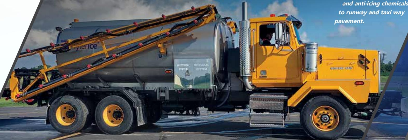
*The Tyler Runwar De-Icer is used to apply de-icing and anti-icing chemicals to runway and taxi way pavement.*
